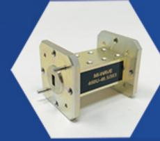
FREQUENCY RANGE: 40.5-50 GHZ REJECTION LEVEL: 40dBC TYP. @ 39.995GHZ PASSBAND INSERTION LOSS: 1.5 dB TYP. INPUT AND OUTPUT PORT: WR19 WAVEGUIDE, UG-383 FLANGE
