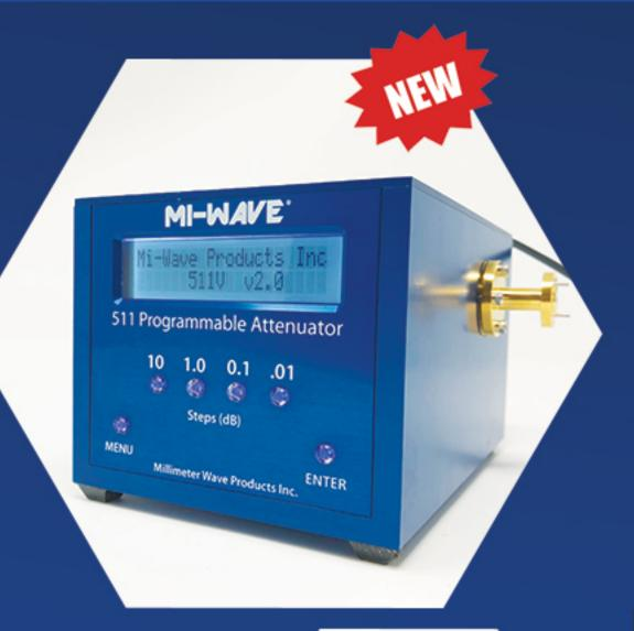
Mi- Wave's 511 Series Precision Programmable Rotary Vane Attenuators are available in full waveguide bands from 7.0 to 220GHz. Attenuation control is performed manually via a front panel or remote controlled using a standard IEEE-488 or USB interface. The attenuators small compact size incorporates both the electronic controller and the microwave components. The unit operates from a single +24 Volt DC source or with an optional adapter.
